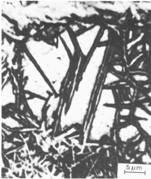
Figure 3 As in Fig. 2, showing coarse and acicular crystals of martensite which appear having been nucleated and grown starting from grain boundaries of the matrix.
