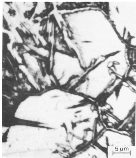
Figure 2 Tapered section of the white layer shown in Fig. 1: a darker phase segregated at grain boundaries of the matrix.
